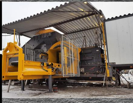
Fully automatised proses creates rectangle wrapped bale independently since the material is loaded into the balers hopper.
